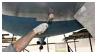
Aplicar High Protect a rodillo
